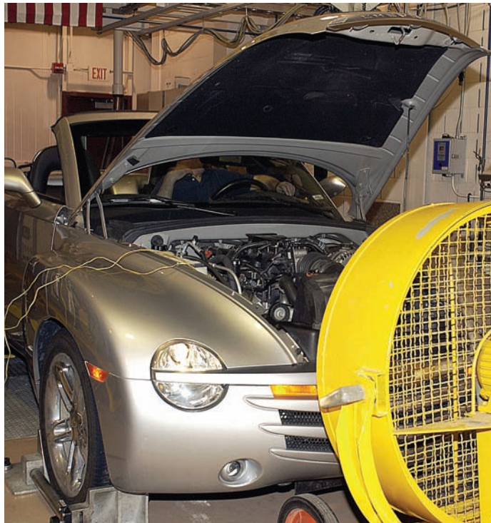
A Chevrolet SSR goes through the FTP regime on a dynamometer at Milford, while sensors record every change in speed and power. GM is performing 500 FTP tests to amass fuel economy data.
