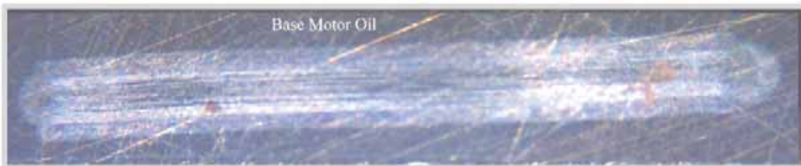
Figure 2. Image of the wear scar on disk for SRV Test No. 1. The mirror finish and the removal of the surface features of the disk, i.e. the deep etching marks, are evidence of polishing wear.
